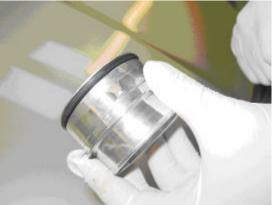
Fit the new hose couplings into their respective fittings on the original intercooler and the turbo outlet pipe on the right side running alongside the engine. Make sure the spring clips are located securely to prevent these couplings from being blown out of the fixings under boost.
