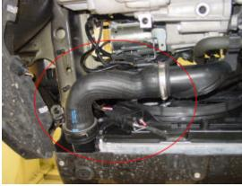
Remove the doubled o-ring seals from the original intercooler hoses and fit these to the included corresponding new aluminium hose couplings as pictured below.
